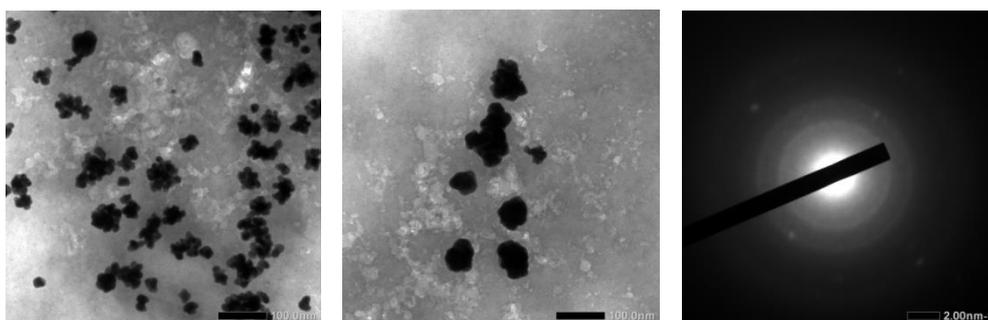
Figure 3: TEM pattern of AuNPs using aqueous extract of *P. obtusifolia* R.Br leaves
